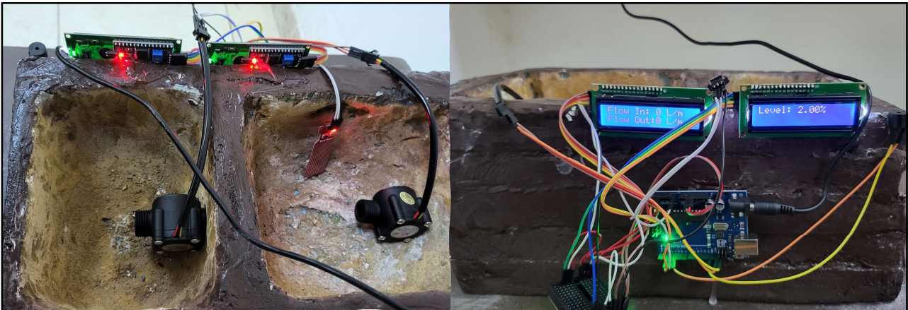
Dam sensors and IoT Flow Units and Water Level Alert System
